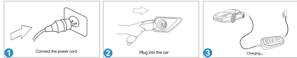
1. Firmly insert the power plug into outlet. Ensure the socket is rated to a current of 10Amp. The Power Green LED light will illuminate
